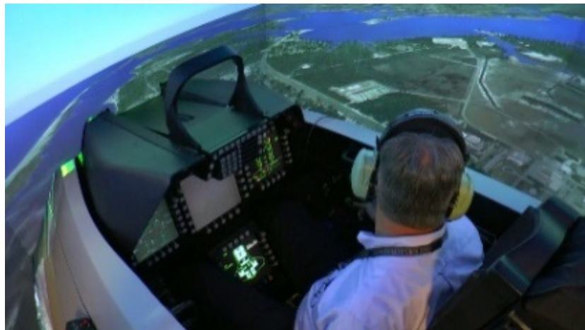
An F-22 Raptor simulator equipped with Boeing's Constant Resolution Visual System at Tyndall U.S. Air Force Base.
